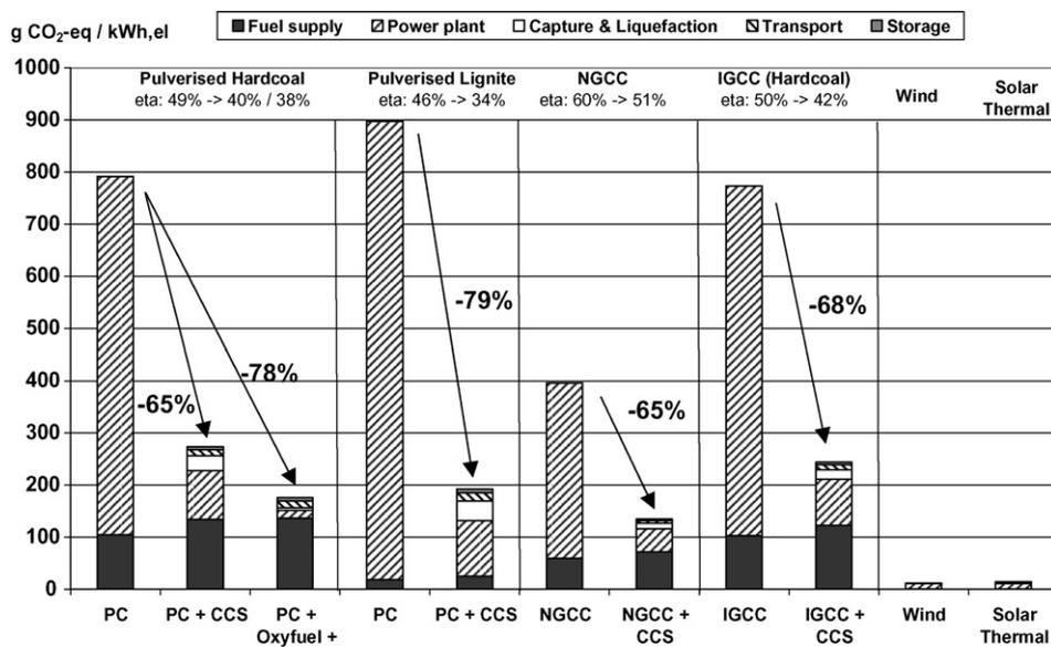
**Fig. 4 – Comparison of greenhouse gas emissions (measured as GWP 100) for pulverised coal power plants (PC), an NGCC, and an IGCC (each of them excluding CCS and including CCS with a CO<sub>2</sub> capture rate of 88% for post- and pre-combustion and of 99.5% for oxyfuel combustion), and renewables (wind offshore, solar thermal electricity).**
