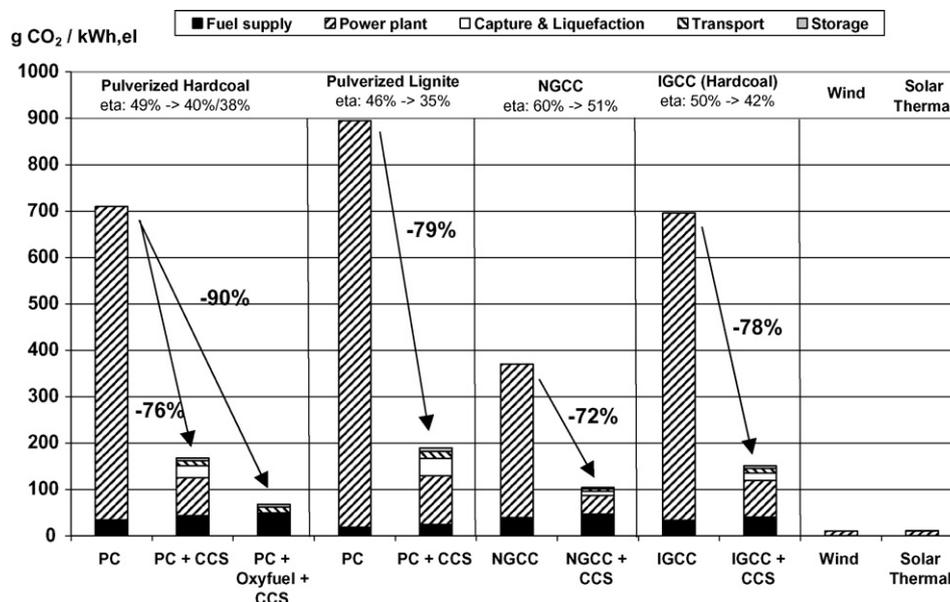
**Fig. 3 – Comparison of CO<sub>2</sub> emissions for pulverised coal power plants (PC), an NGCC, and an IGCC (each of them excluding CCS and including CCS with a CO<sub>2</sub> capture rate of 88% for post- and pre-combustion and of 99.5% for oxyfuel combustion), and renewables (wind offshore, solar thermal electricity).**
