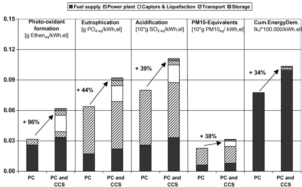
**Fig. 5 – Further impact categories illustrated by way of the pulverised hard coal power plant (CO<sub>2</sub> capture rate of 88%).**
