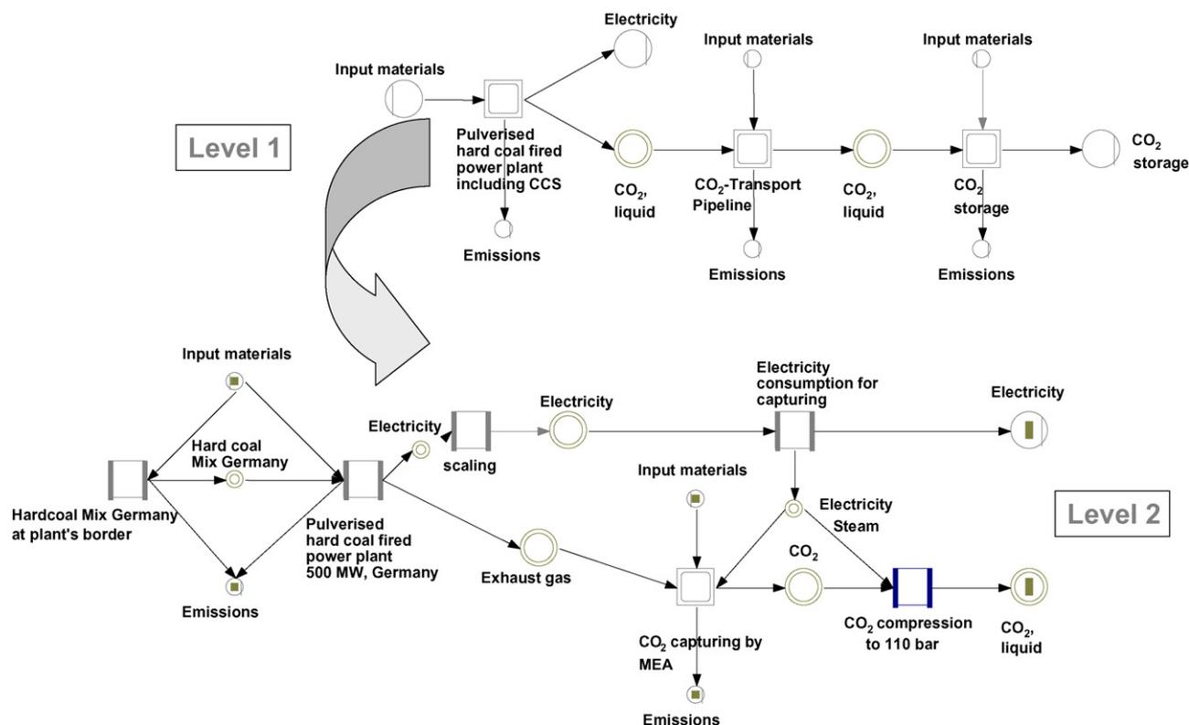
Fig. 1 – Material and energy flow network of a coal-fired power plant including CO<sub>2</sub> capture and storage.
