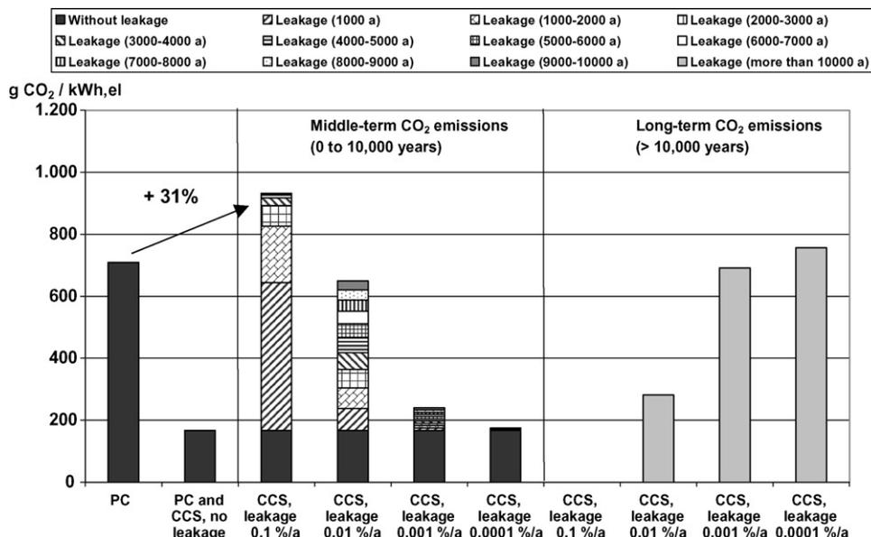
**Fig. 7 – Sensitivity analysis 2: assuming different storage leakage rates (0.1–0.0001%/a). Comparison of middle-term and long-term release of carbon dioxide by way of the pulverised hard-coal power plant (CO<sub>2</sub> capture rate of 88%).**
