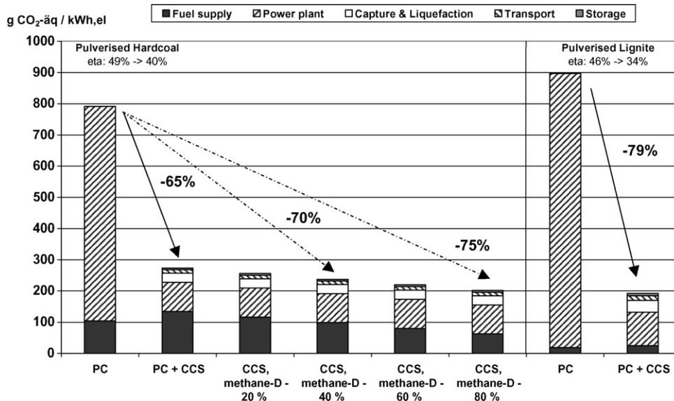
**Fig. 6 – Sensitivity analysis 1: greenhouse gas emissions of a hard coal-fired power plant depending on a change of the methane emissions from hard coal mining and comparison with a lignite-fired power plant (each of them with a CO<sub>2</sub> capture rate of 88%).**
