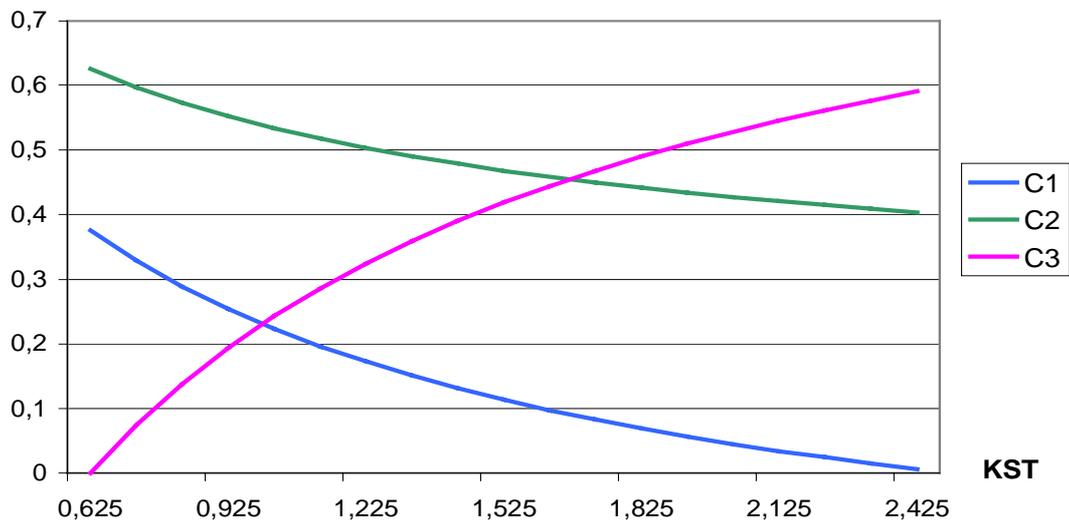
**Fig. 2.26** Coefficients  $C_1$ ,  $C_2$  and  $C_3$  as functions of parameter  $KST$  as used to calculate flow routing with the Muskingum equations 182-184 assuming that  $X = 0.2$  and  $\Delta t = 1$
