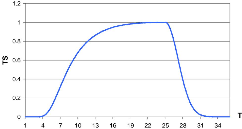
**Fig. 2.10** Temperature stress factor as a function of average daily air temperature (equations 96 and 98), assuming  $T_O = 25^\circ \text{C}$  and  $T_B = 3^\circ \text{C}$
