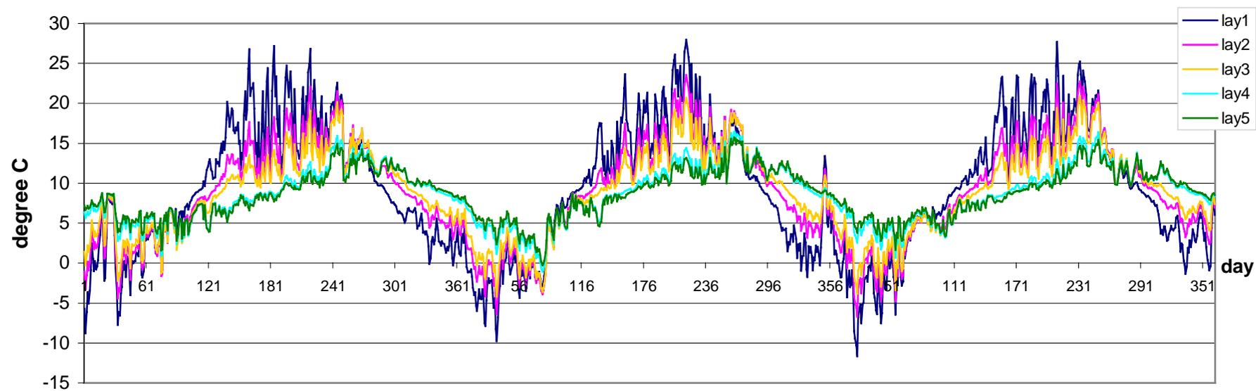
**Fig. 2.18** An example of soil temperature dynamics in five soil layers simulated with SWIM using equation 131
