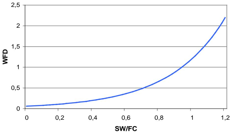
**Fig. 2.20** Soil water factor of denitrification (equation 151)
