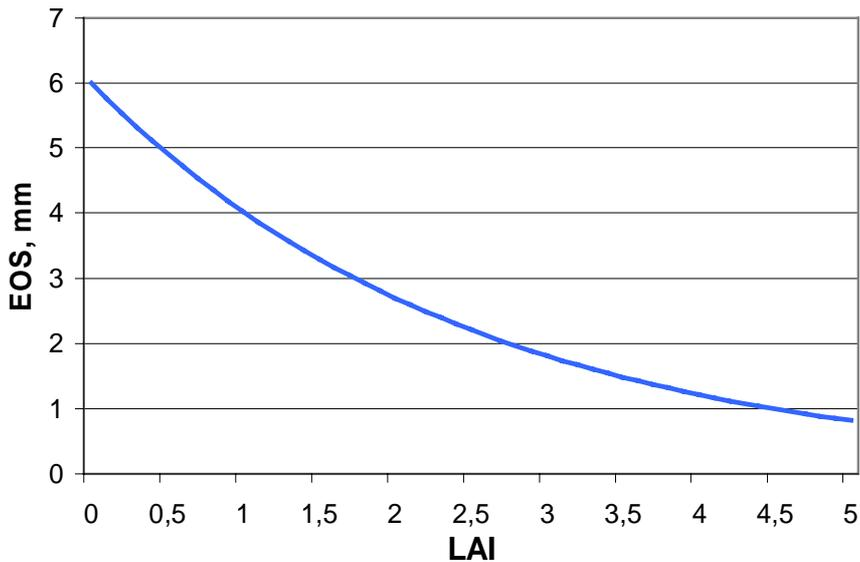
**Fig. 2.7** Potential soil evaporation,  $ESO$ , as a function of leaf area index,  $LAI$  (equation 61) under assumption that  $EO = 6 \text{ mm d}^{-1}$
