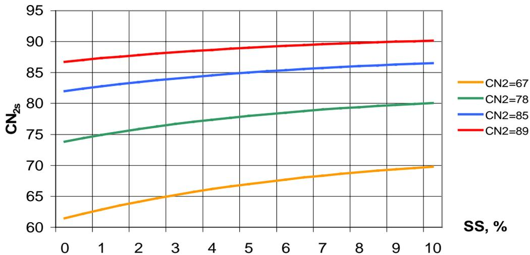
**Fig. 2.3** Adjustment of curve number  $CN_2$  to the slope (equation 8) for some typical values of  $CN_2 = 67, 78, 85,$  and  $89$ , corresponding to straight row crop and four hydrologic groups A, B, C, and D, respectively
