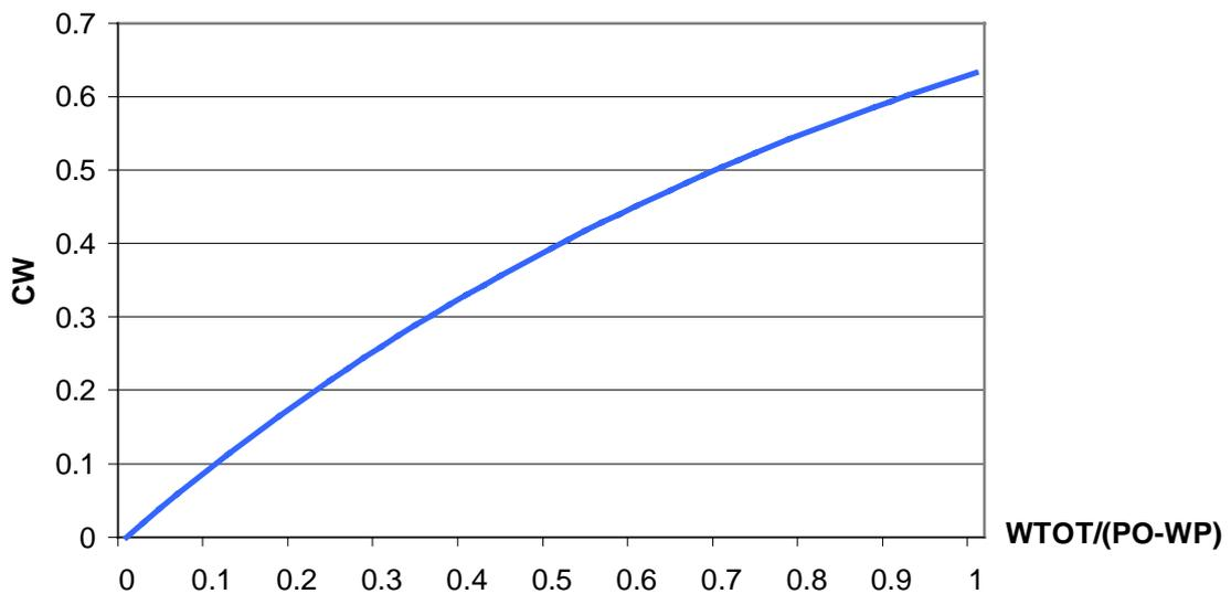
**Fig. 2.22** Coefficient  $CW$  to calculate the amount  $NO_3$ -N lost from the layer as a function of water content (equation 160)
