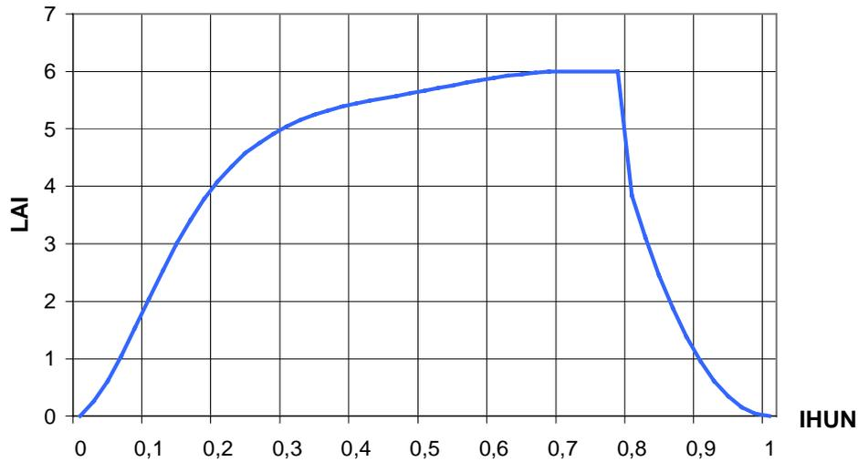
**Fig. 2.9** Leaf area index as a function of the heat unit index (equation 87)
