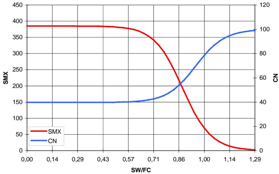
**Fig. 2.4** Retention coefficient SMX and curve number CN as functions of soil water content SW (equation 9 and 4) assuming  $CN_2 = 60$ ,  $WP = 5 \text{ mm mm}^{-1}$ ,  $FC = 35 \text{ mm mm}^{-1}$ ,  $PO = 45 \text{ mm mm}^{-1}$
