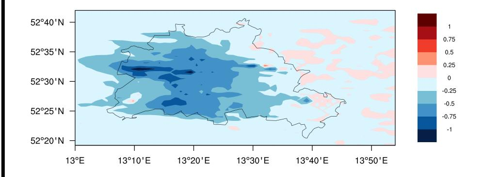
**Figure 9:** Temperature differences in Berlin, 2003-08-10 12pm CET (noon), when simulated with a roof albedo of 0.65 compared to the albedo of the reference simulation of 0.18 in fig. 7
