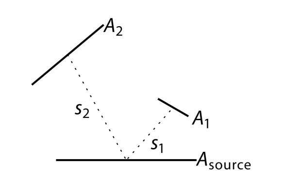
**Figure 3:** Averaging of street widths. In this example, the distances s<sub>1</sub> and s<sub>2</sub> between the "source area" and the "receiving areas" are weighted by  $A_1$  and  $A_2$ , respectively.
