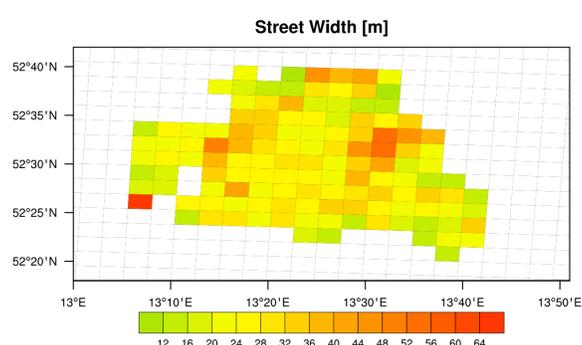
**Figure 5:** Street width  $W$  for canyons with a north-south direction in Berlin calculated from the average distance of wall surfaces.
