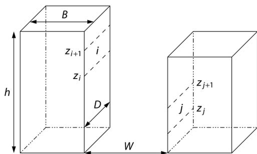
**Figure 1:** building width  $B$ , street width  $W$ , canyon length  $D$ , probability  $\gamma(h)$  of building height  $h$ ; also: canyon angle  $\chi$  relative to north-south direction, urban fraction  $F$  of a cell
