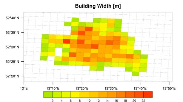
**Figure 6:** Building width  $B$  for canyons with a north-south direction in Berlin calculated from  $B = A_B W / (F - A_B)$ .
