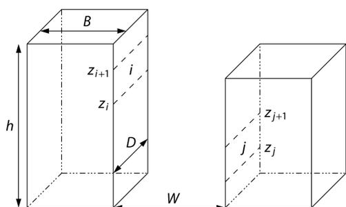
Figure 1: Basic urban street canyon model (Martilli et al. 2002)
