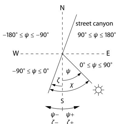
Figure 2: The angle  $\chi$  between the urban street canyon and the sun is calculated from the street direction  $\zeta$  and the solar azimuth  $\psi$ .
