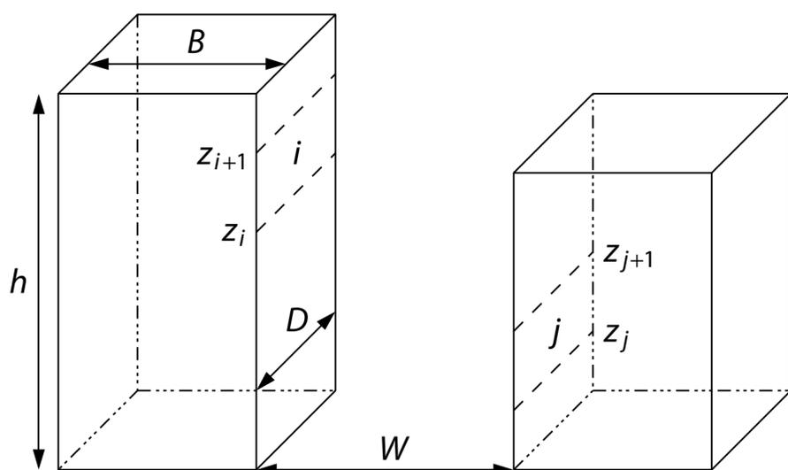
**Figure 1:** Basic urban street canyon model (Martilli et al. 2002): **building width**  $B$ , **street width**  $W$  and **canyon length**  $D$ . For every grid cell, the **distribution of the height**  $h$  of the building is given by  $\gamma(h)$ . The urban layer is divided in several height levels  $i$ . Further parameters: **canyon angle**  $\chi$  relative to north-south direction, **urban fraction**  $F$  in a grid cell.
