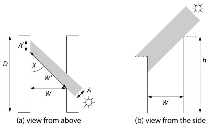
**Figure 2:** Visualization of the effective sunlit wall surface  $A'$  and canyon width  $W'$  in (a) and the shade effect in (b)
