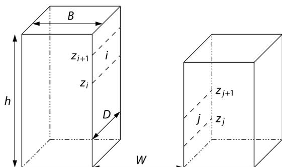
**Figure 1:** Basic urban street canyon model (Martilli et al. 2002): canyon width  $D$ , building width  $B$ , street width  $W$  and canyon length  $D$ . For every grid cell, the distribution of the height  $h$  of the building is given by  $\gamma(h)$ . The urban layer is divided in several height levels  $i$ .
