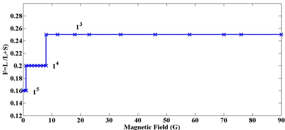
FIG. 11. Devil's staircase represents the changes in the firing number with the magnetic field at 240 V.
