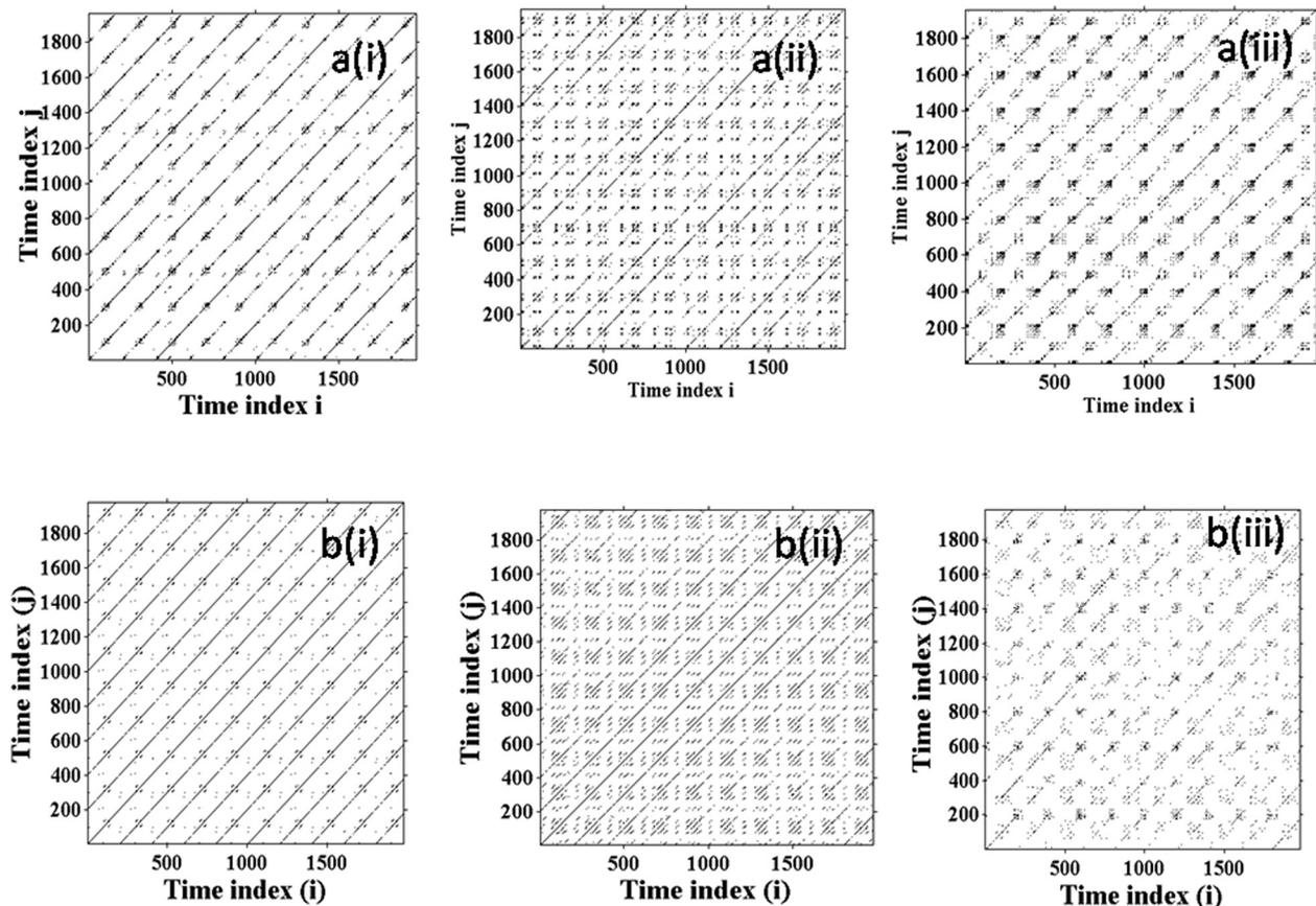
FIG. 6. (a) and (b) Recurrence plot of the floating potential fluctuations obtained in (i) regime I, (ii) regime II, and (iii) regime III at (a) 250 V and (b) 240 V with  $B = 0$ .
