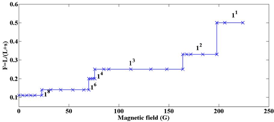
FIG. 10. Devil's staircase shows the variation in the firing number with the magnetic field at 250 V.
