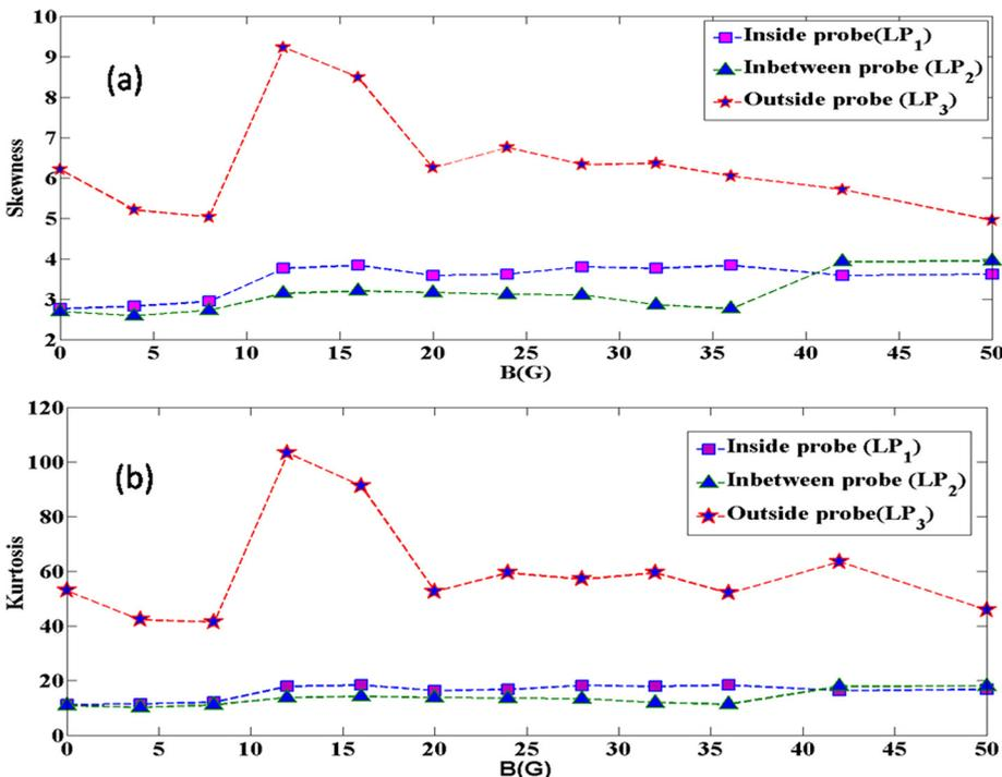
FIG. 9. (a) Skewness and (b) kurtosis of the floating potential fluctuations in different magnetic fields at 240 V.
