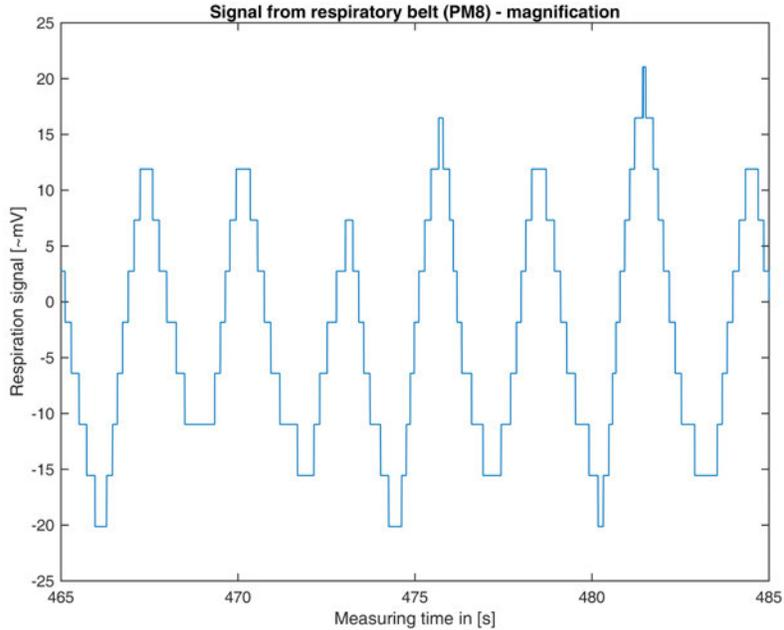
Figure 1: Signal from respiratory belt (PM8) - magnification. There is a visible formation of steps due to a wrong amplitude quantisation (too little amplification of the signal for given resolution).
