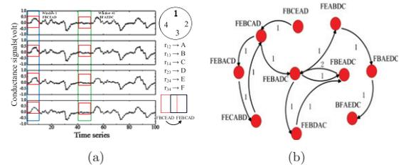
Fig. 4: (Colour online) (a) Schematic diagram for the construction of a directed weighted complex network from multivariate time series. (b) Topological structure of the complex network generated from the multivariate time series shown in (a). Figure from ref. [102].
