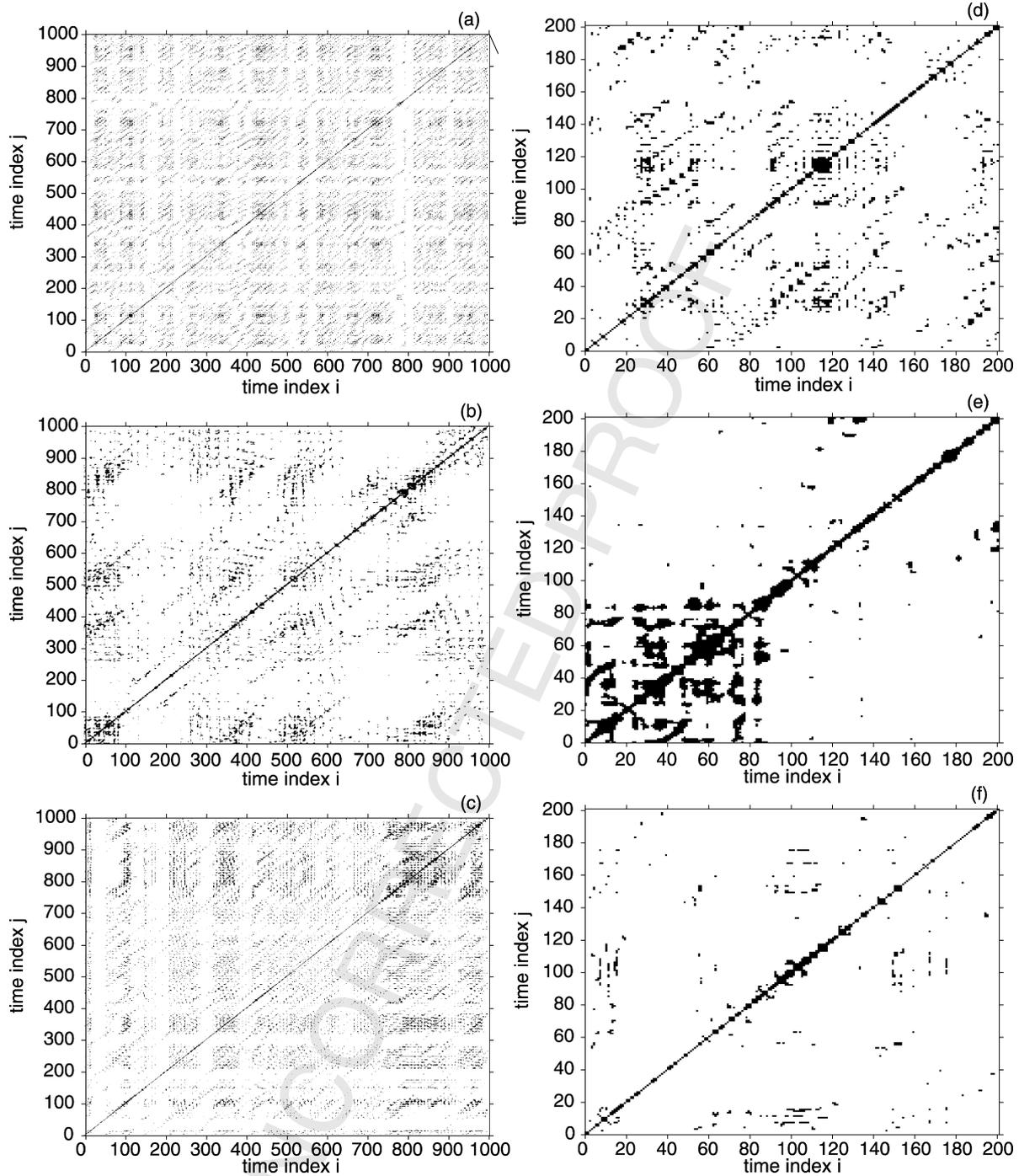
Fig. 3. Recurrence plots for the first 1000 points (corresponding to a 1 ms time window) of the series for floating potential for radial positions (a)  $r = 16.5$  cm, (b)  $r = 18.0$  cm, and (c)  $r = 21.0$  cm. Magnifications of the lower left corners of these plots are shown in (d), (e), and (f), respectively.
