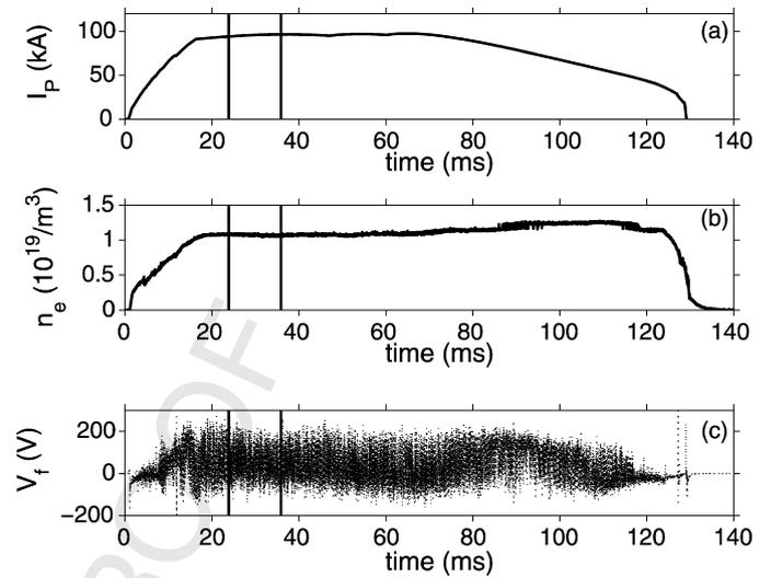
Fig. 1. Time evolution of (a) plasma current, (b) electron density, and (c) floating potential for a typical discharge of TCABR tokamak. The vertical lines indicate the time window used in recurrence quantification analysis.
