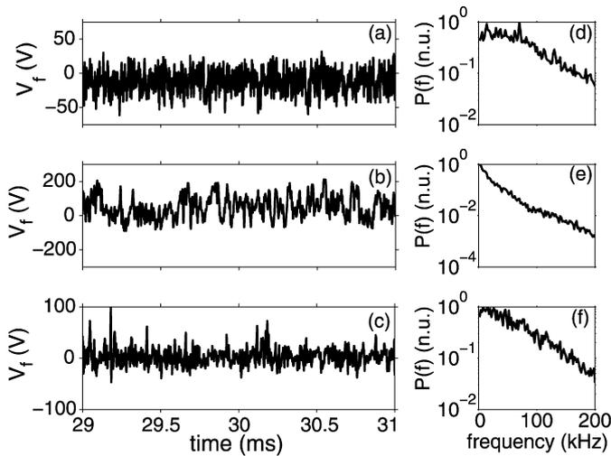
Fig. 2. Time evolution of the floating potential measured by Langmuir probes placed at radii (a)  $r = 16.5$  cm, (b)  $r = 18.0$  cm, and (c)  $r = 21.0$  cm. The corresponding power spectral densities are depicted in (d), (e), and (f), respectively.
