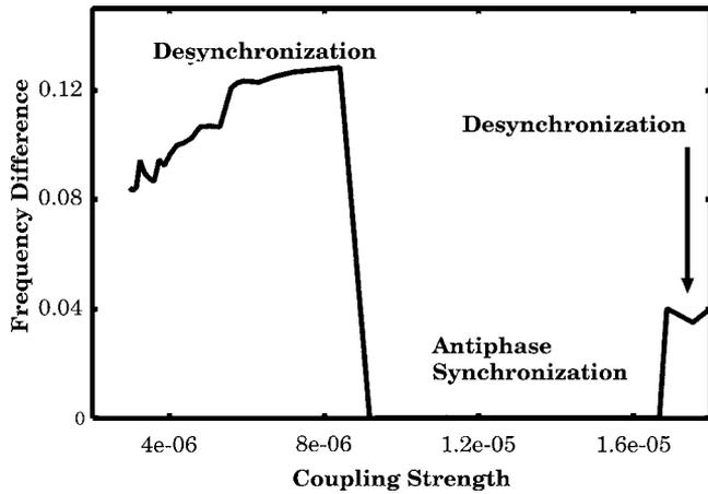
FIG. 9. Synchronization diagram of two diffusively coupled nonidentical Chua circuits. Frequency difference  $\Delta\omega$  between the two circuits is plotted against coupling strength  $C=1/R_c \in [0, 1.8 \times 10^{-5}]$ .
