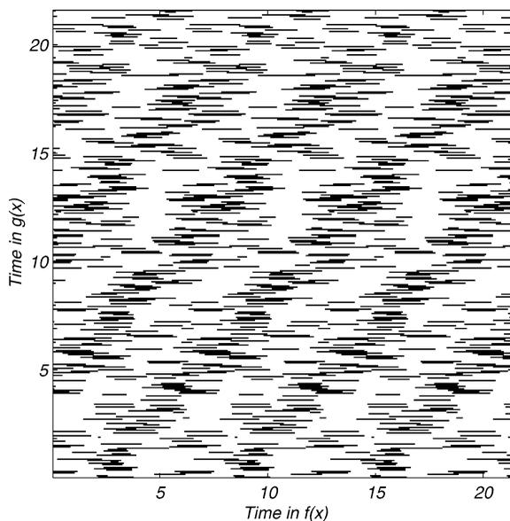
Fig. 2. Cross recurrence plot for two delayed sine functions (Fig. 1) with an embedding of  $m = 3$ ,  $\tau = \pi/2$  and  $\varepsilon = 1.5$ . The diagonal lines in the CRP result from similar phase space behaviour of both functions.
