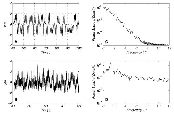
Fig. 4. (B) Time series of a nonlinear related system consisting of a driven first order autoregressive process, forced by the squared (A) *x*-component of the Lorenz system ( $\kappa = 0.2$ ). The major periods (frequencies) are 2.9 (0.34) and 1.1 (0.94) for *x* (C) and 0.77 (1.30) and 0.96 (1.05) for *y* (D).
