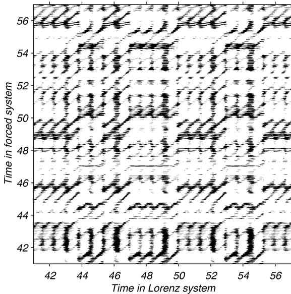
Fig. 5. Cross recurrence plot for the forced autoregressive process  $y$  (Fig. 4B) and the forcing function ( $x$ -component of the Lorenz system, Fig. 4A) for a coupling strength  $\kappa = 0.2$  and an embedding  $m = 5$ ,  $\tau = 10$ ,  $\varepsilon = 2$ .
