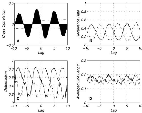
Fig. 3. Cross-correlation (A), *RR* (B), *DET* (C) and *L* (D) for two delayed sine functions. *L* has the unit of time. The solid black lines show positive relation, the dashed lines show negative relation. The dash-dotted line in (A) marks the 5% confidence interval. All functions (A)–(D) detect the correlation after a lag of  $\pi/2$ .
