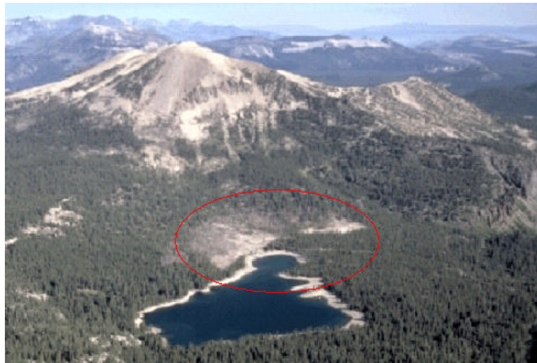
Figure 2.3: Impact of soil outgassing of >1,200\text{t CO}_2 per day in a 30 hectare area on local ecosystems at Mammoth Mountain, California. Source: Friberg [2004].
