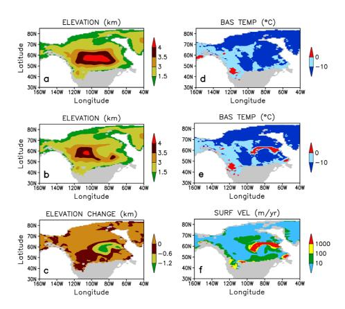
**Figure 3.** Heinrich event VI (in Figure 1) is shown here. Elevation of the LIS (a) before and (b) after that HE. (c) Difference between the elevations before and after the same HE. Basal temperature corrected for pressure melting (d) before and (e) during that HE. (f) Ice-surface velocity during the same HE
