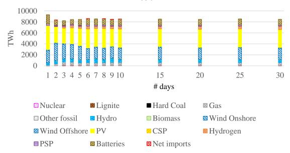
Figure 9. Impact of modelled representative days on the generation-mix at the EU ETS level in 2030 and 2050.
