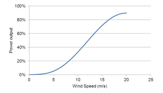
Figure 3. Aggregated wind power curve. Source: Own calculations based on Dee et al. (2011), ÜNB (2013a) and ÜNB
