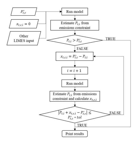
Figure A2. Flow diagram explaining the iterative process formulated to run the model when a minimum CO<sub>2</sub> price is
