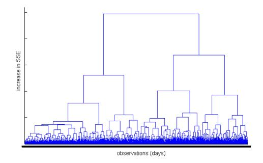
Figure 2. Dendrogram of clustering procedure. Showing the consecutive grouping of two clusters to a joint cluster and the resulting increase in the overall sum of squared errors (SSE, y-axis). All days (x-axis) are consecutively grouped together until only one cluster is left. Source: Own computation with model-specific data.
