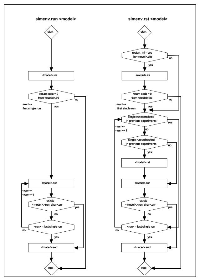
Fig. 7.1 Flowcharts for performing simenv.run and simenv.rst
