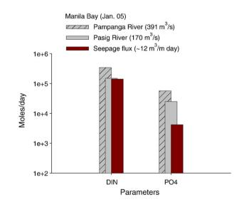
Fig. 10–Estimated fluxes of dissolved inorganic nitrogen (DIN) and PO<sub>4</sub> via SGD and from the two most important rivers draining into Manila Bay (data from Taniguchi et al., 2008).
