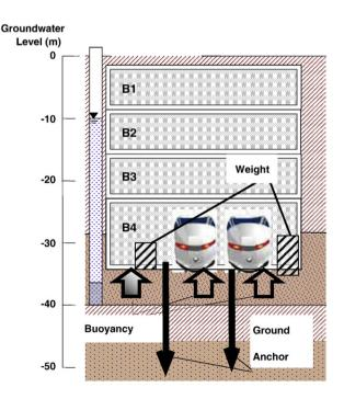
Fig. 5–Procedures against buoyancy due to increase in groundwater level using weight and ground anchor (Aichi et al., 2006).
