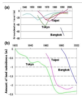
Fig. 4–Change in (a) groundwater level and (b) amount of subsidence.
