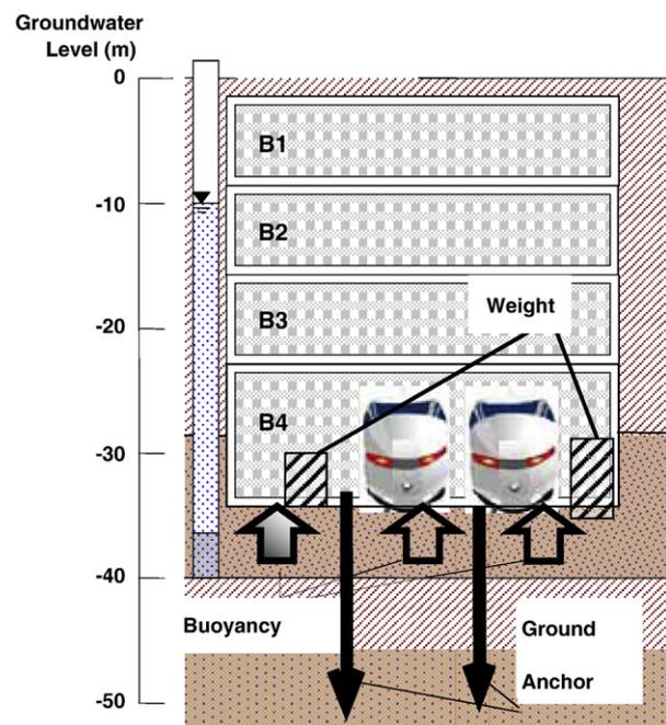
Fig. 5—Procedures against buoyancy due to increase in groundwater level using weight and ground anchor (Aichi et al., 2006).
