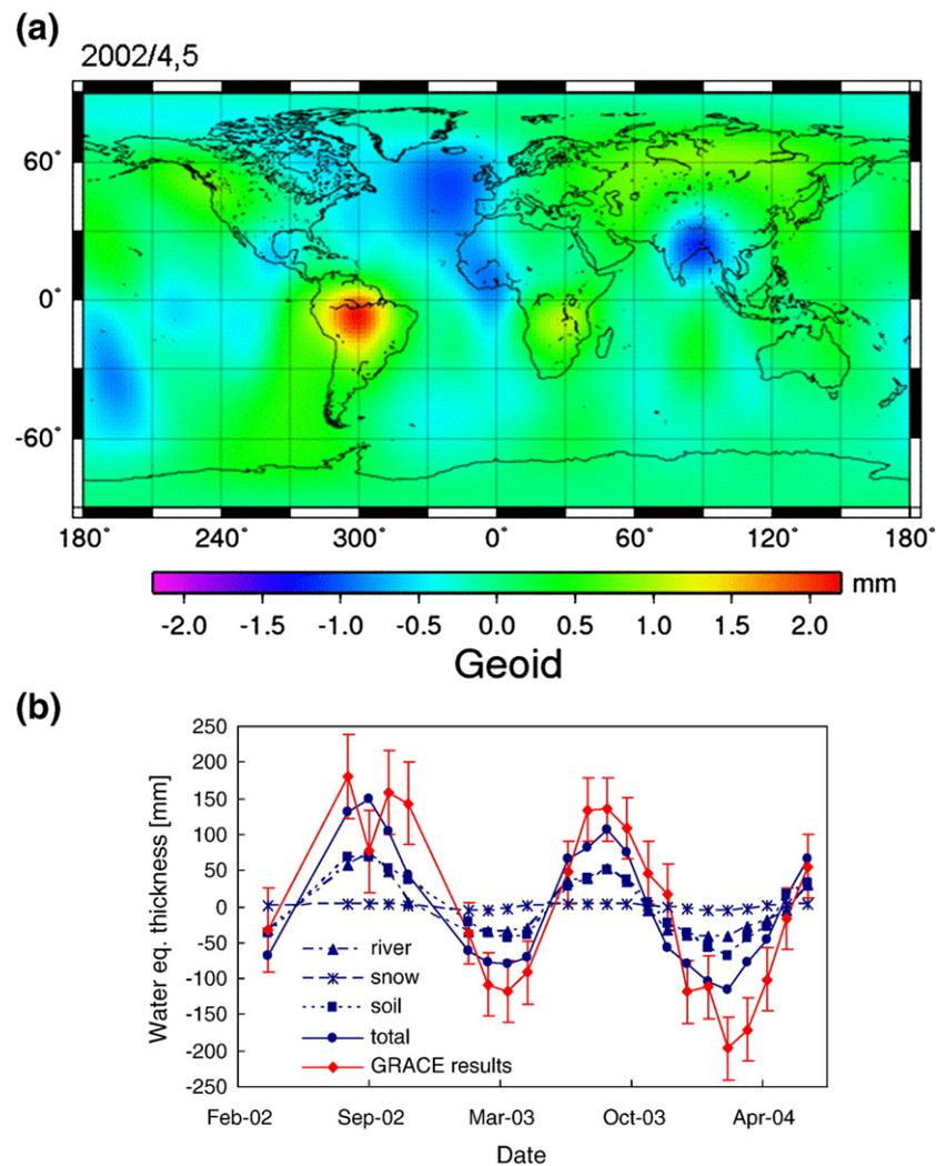
**Fig. 8 – Gravity anomalies obtained from (a) GRACE for April and May 2002 with mean radius of 1000 km (Fukuda et al., 2005), and (b) comparisons of GRACE and model data for four river basins (Chao Phraya, Mekong, Salween and Irrawaddy) (Fukuda et al., 2005).**
