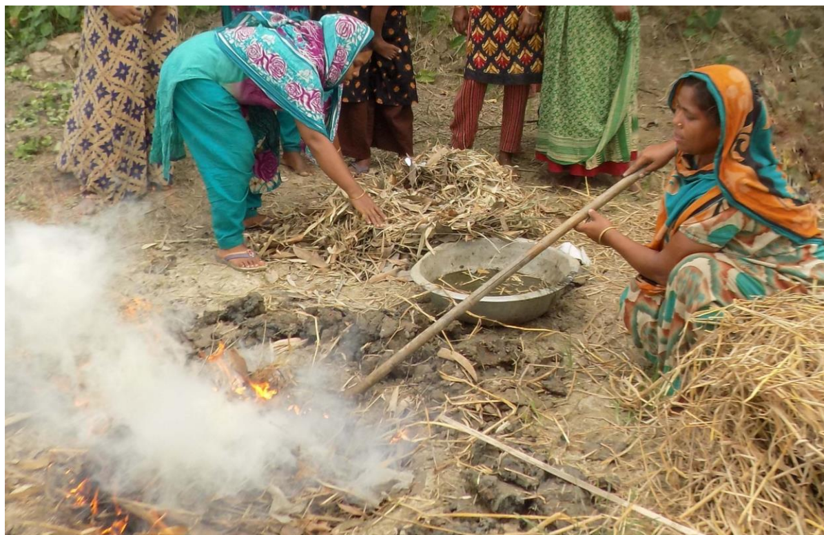
Too much feedstock was added at once to the kiln, causing smoke.
