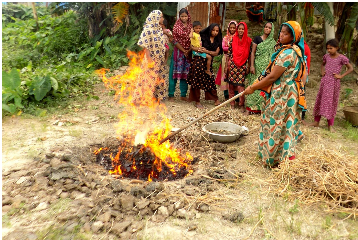
No smoke, and the material in the kiln is black. Good production!
