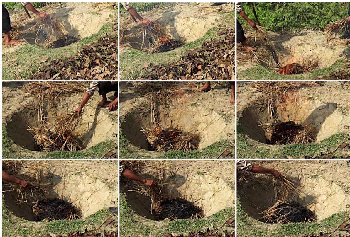
Adding biomass piece by piece as the previous biomass is pyrolysed.
