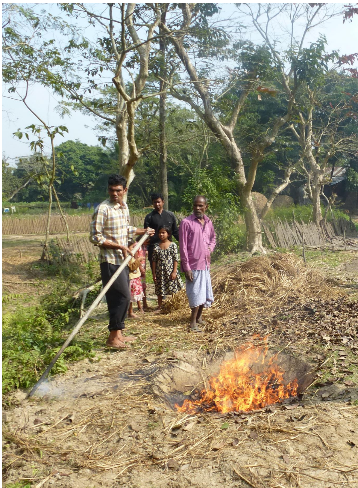
The kiln is not full at the time of firing and a large amount of feedstock is reserved.
