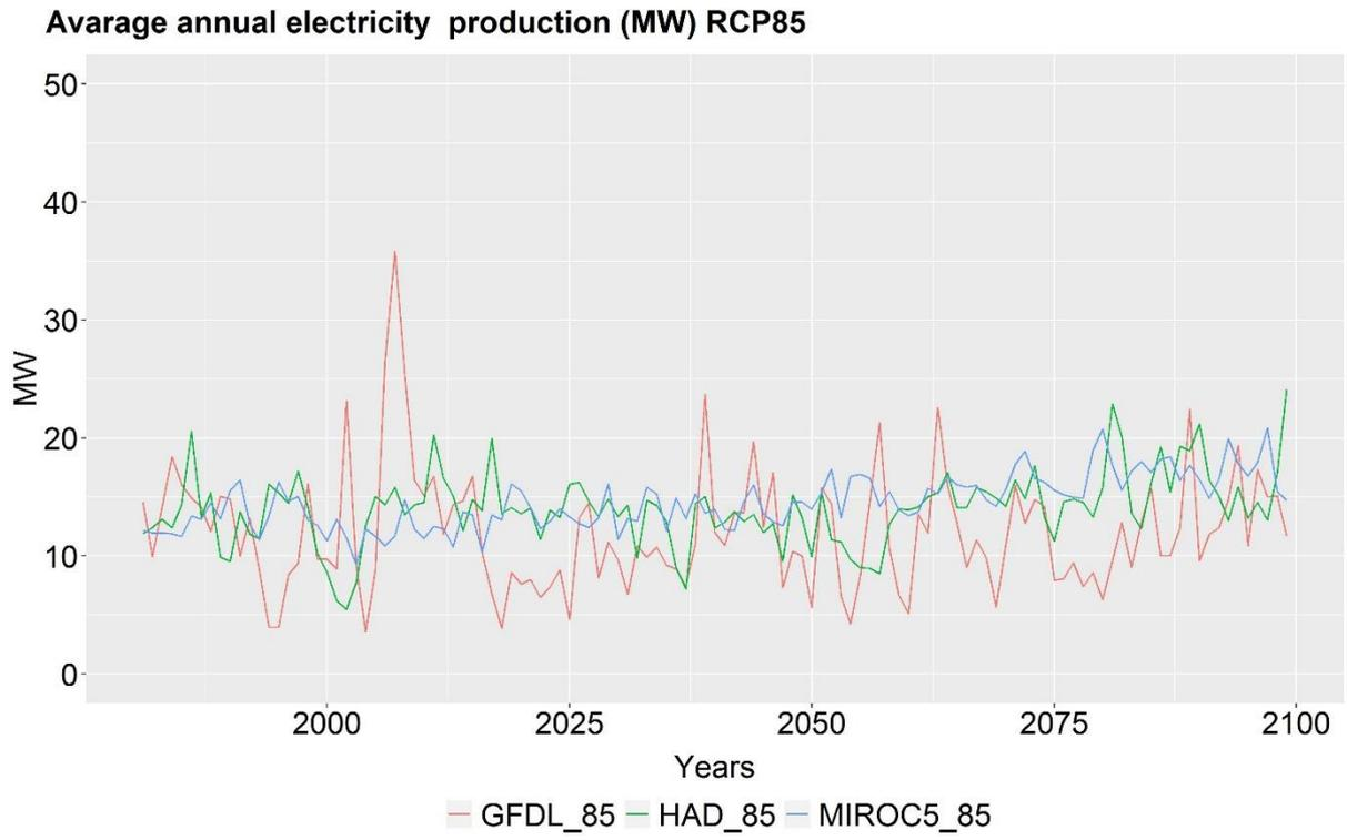
Figure 12 Annual average electricity production of the Koka (Awash 1) HPP under RCP 8.5 to the end of the century
