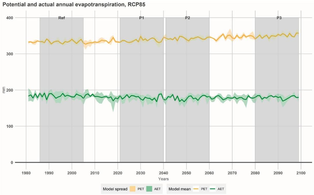
Figure 10 The multi-model mean of annual potential and actual evapotranspiration under RCP 8.5 to the end of the century
