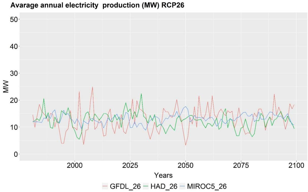
Figure 11 Annual average electricity production of the Koka (Awash 1) HPP under RCP 2.6 to the end of the century
