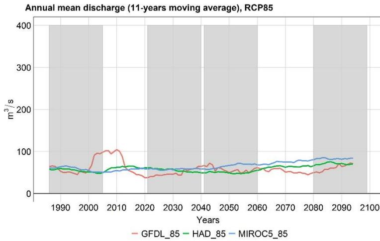
Figure 6 Annual mean discharge at the Hombole gauge (11-years moving average) under RCP 8.5
