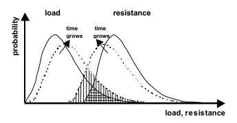
**Figure 3.** Load-resistance analogy in a changing world.
