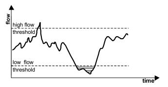
Figure 1. Definitional sketch of threshold crossing.
