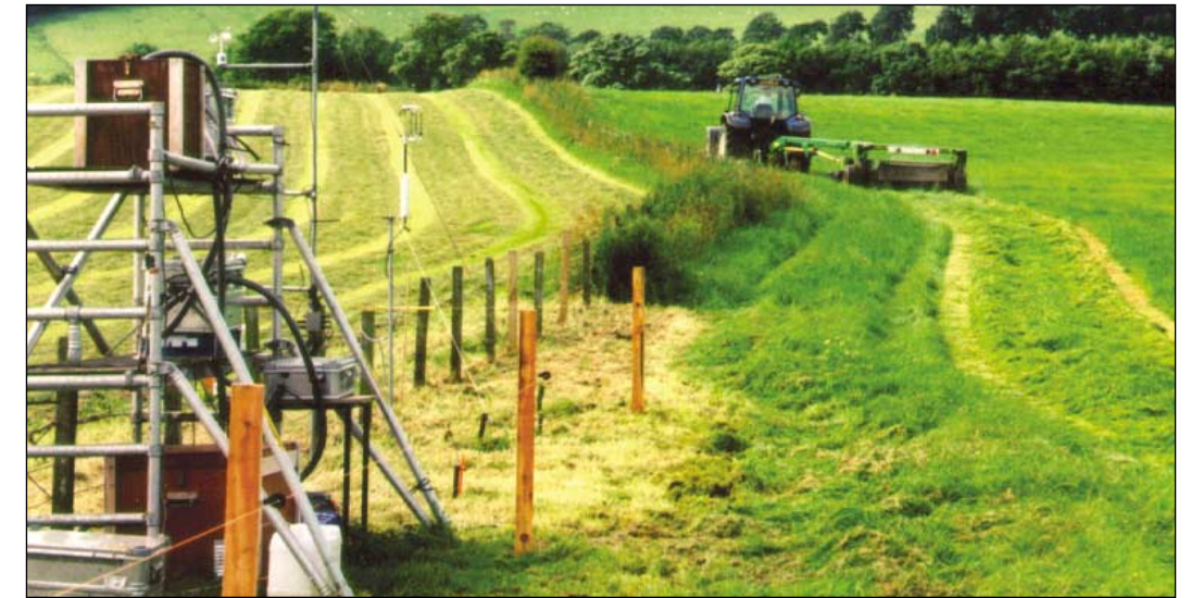
Figure 9.2a Equipment to measure ammonia exchange located over a managed grassland.
