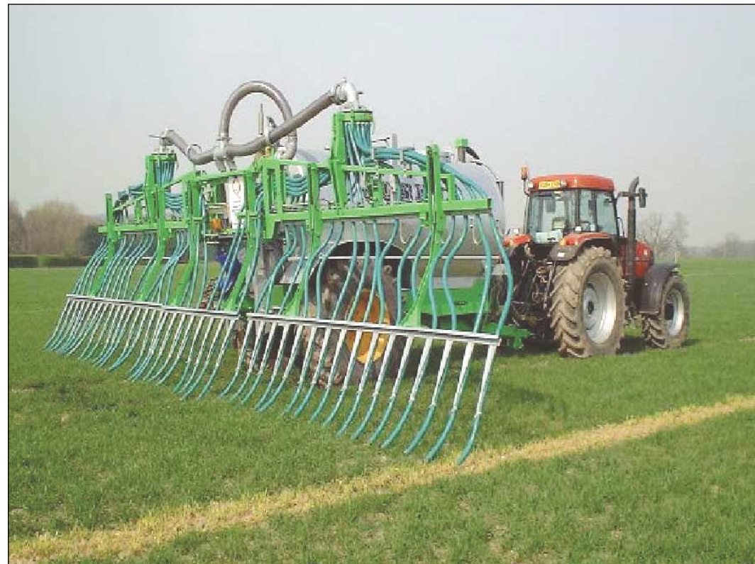
Figure 6.3 Top dressing a crop with pig slurry using a trailing hose boom.
