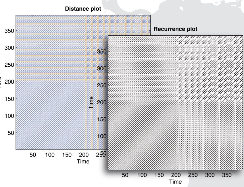
Distance plot (left) of the Rössler system. In order to construct a recurrence plot from a phase space trajectory, a threshold is applied on the distance plot. Corresponding recurrence plot (right) of the considered system. The transition from periodic to chaotic behaviour is obvious.
