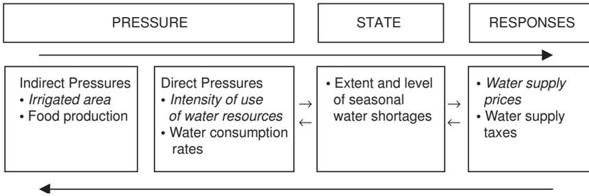
**Figure 14.3** Water resources pressure-state-responses (P-S-R) model. Italics highlight indicators in the Core Set; others are presented as supplementary or are being further developed. Source: OECD (1998).
