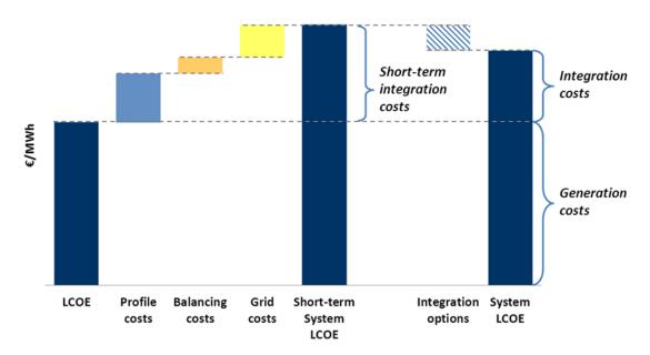
Figure 6: Integration costs are divided into three components: profile, balancing and grid costs. To some extent integration costs that occur in the short term can be reduced by integration options in the long term.
