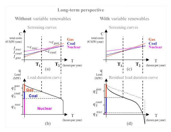
Figure 7 (illustrative): Long-term screening curves and load duration curves without (left) and with wind deployment (right). Wind changes the residual load duration curve (c, d). Thus capacities adjust towards lower fixed-to-variable-costs ratio (more gas capacity, less nuclear capacity).
