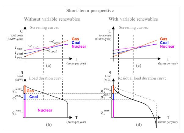
Figure 8 (illustrative): Optimal long-term capacities are derived without VRE (a, b). With VRE the LDC transforms to a RLDC (d). In the short-term perspective the capacities remain unchanged (b, d). Hence, specific costs increase because technologies operate in full-load hour ranges where they would not be cost-efficient if capacities could optimally adjust (c).
